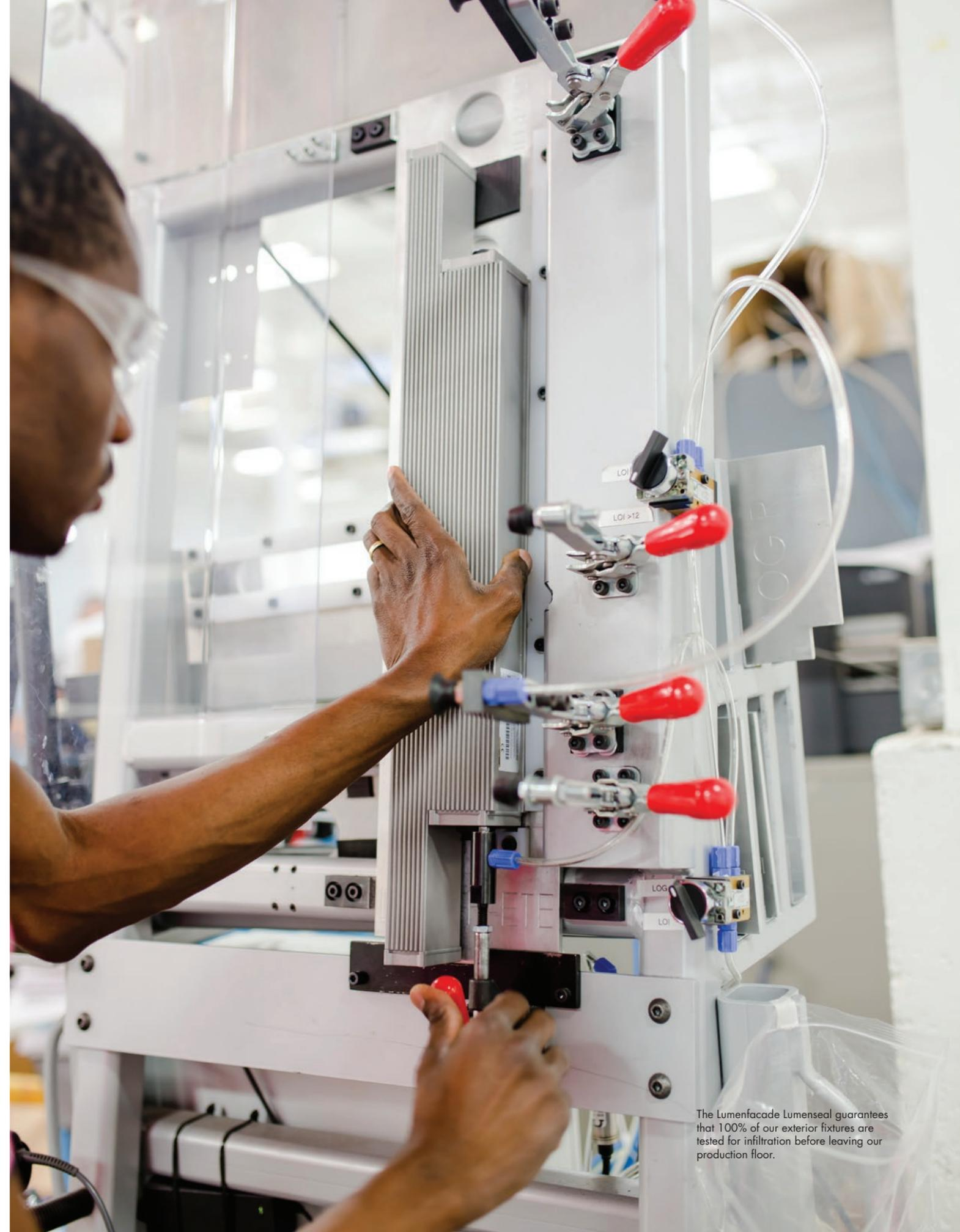
The Lumenfacade Lumenseal guarantees that 100% of our exterior fixtures are tested for infiltration before leaving our production floor.
